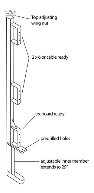
The Perimeter Guardrail Post is now available for purchase. The top adjusting wing nut makes adjustment quick and easy from a standing position.
